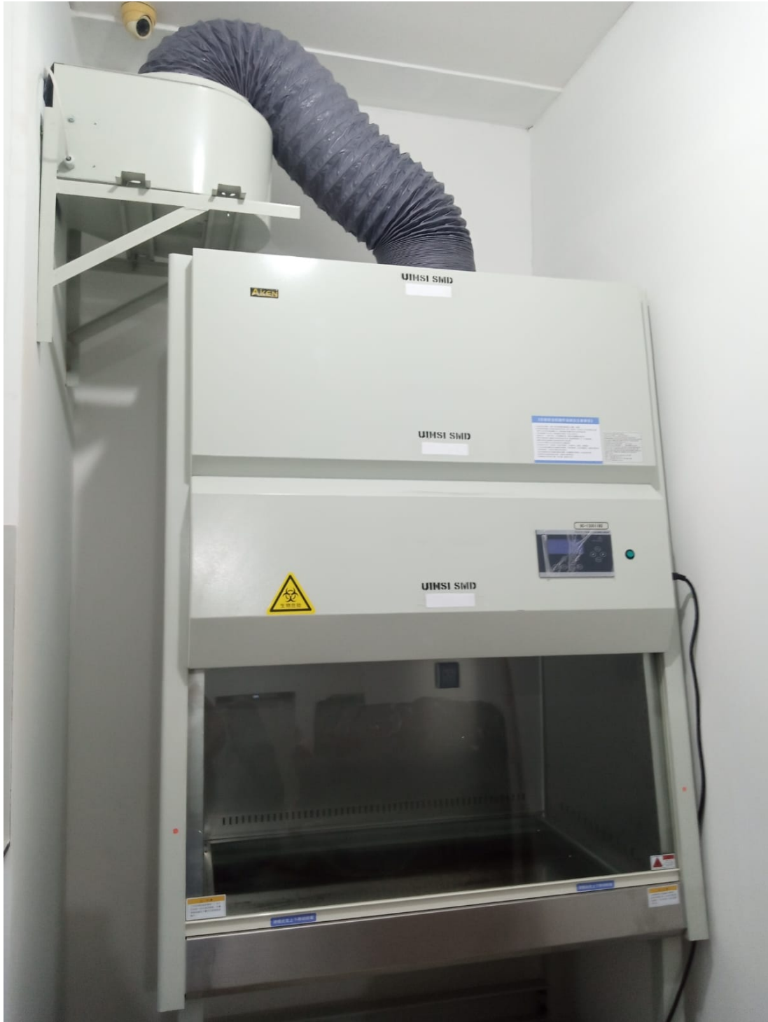
Biology Safety Cabinet
